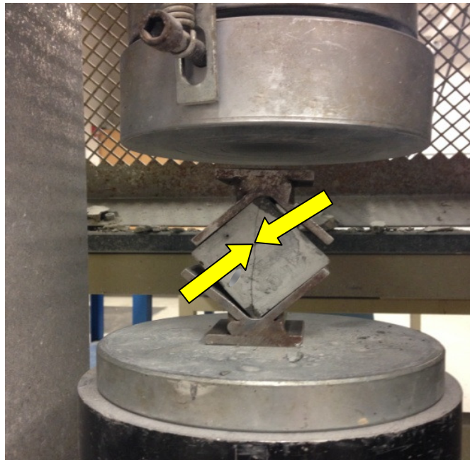
Figure 4: Vertical Crack in Split Tensile Strength Test Cube
