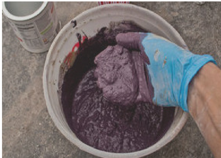
Figure 3: Incorporation of PVA Microfibers in Concrete
