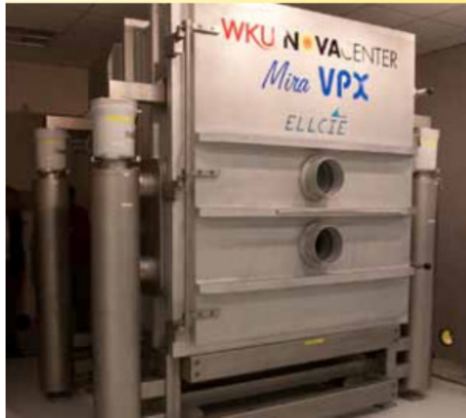
Figure 5: Large Chamber Scanning Electron Microscope at WKU NOVA Center
