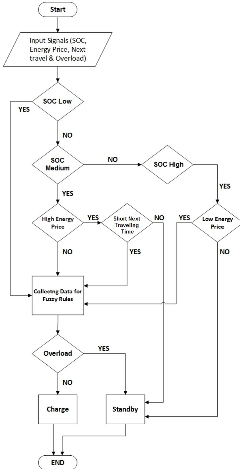
Figure 4: Fuzzy Logic Control System Mechanism
