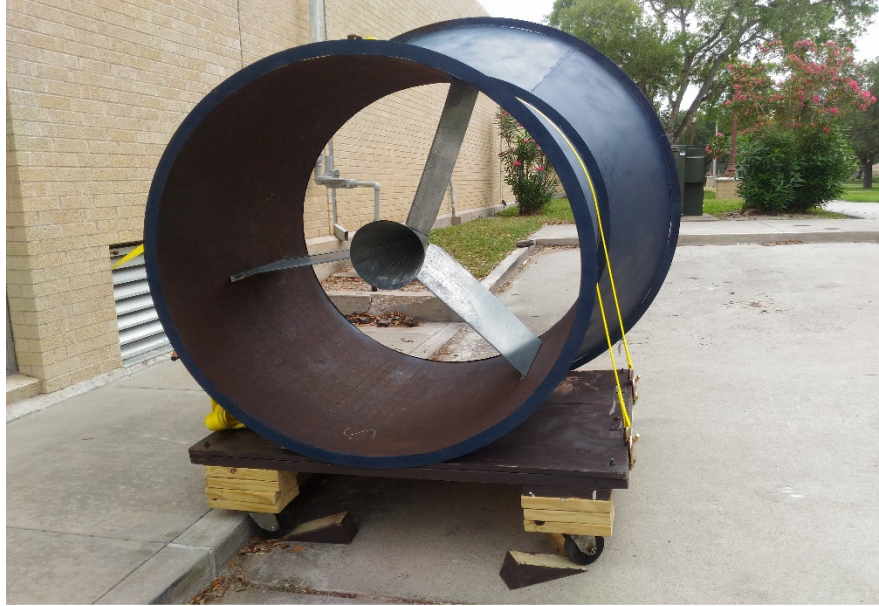
Figure 2 – Wind Augmentation Device With Cone
