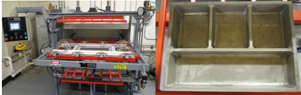
Figure 2. MAAC thermoforming machine and aluminum mold with vacuum holes.
