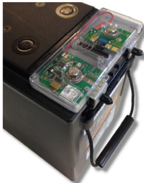
Figure 3. Battery monitor mounted on an UltraBattery.
