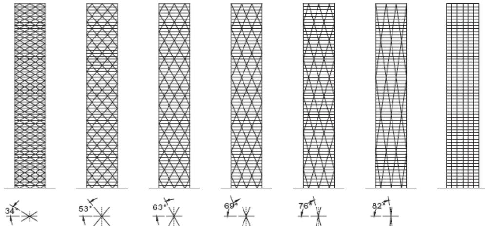
Figure 1: 60-story structures with various diagonal angles to find out optimal angle [1]
