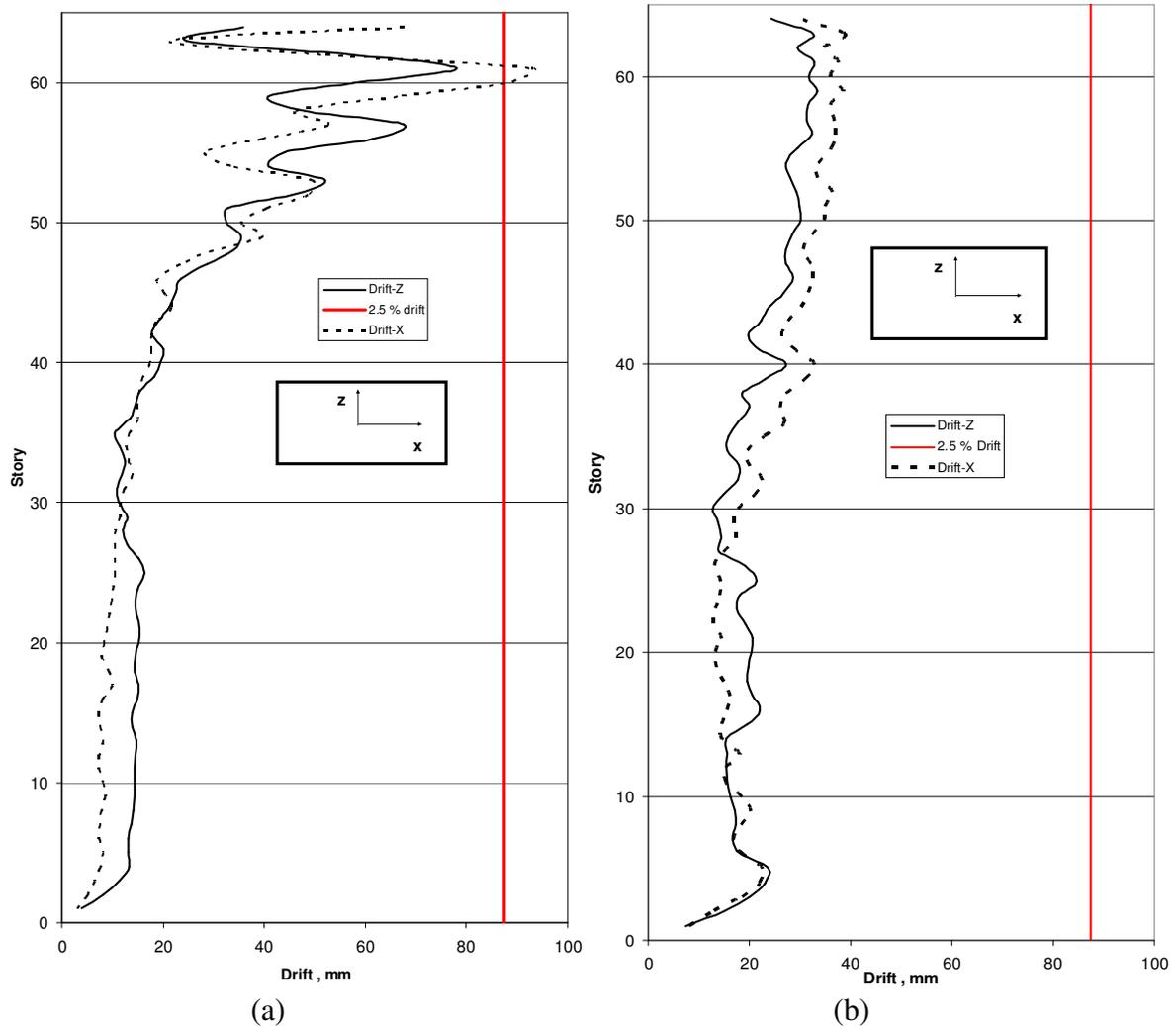
Figure 7: Inter-story drift of the 64-story structure due to Kobe earthquake from (a) Iteration-1; (b) Iteration-2
