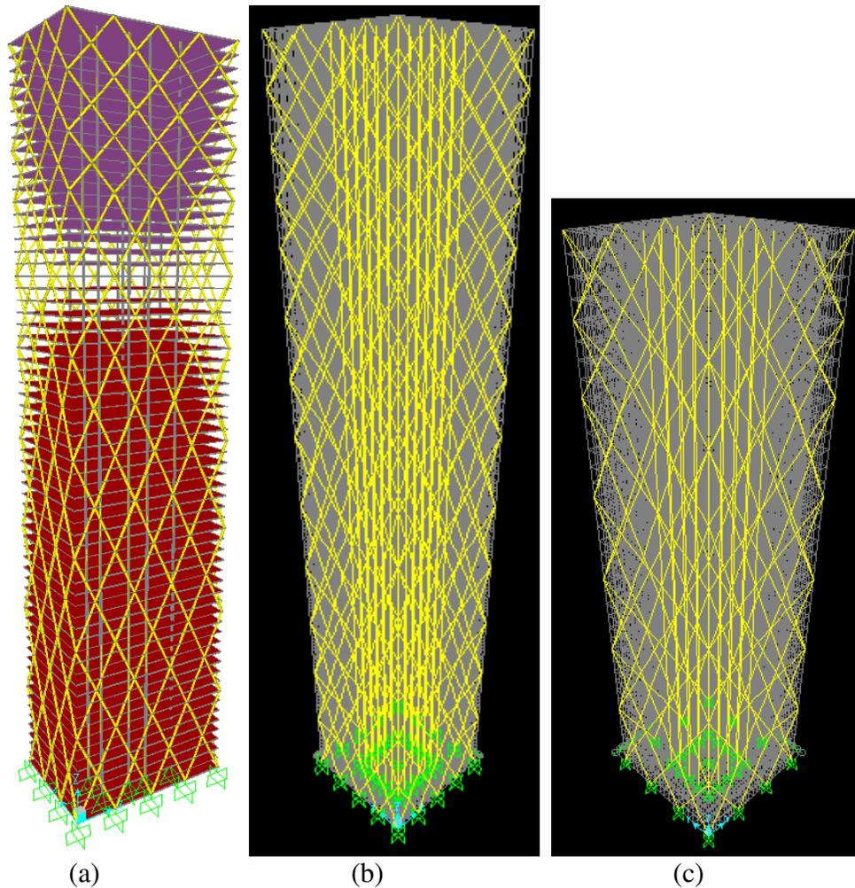
Figure 8: 3-D view of Diagrid structure (a) 64-story; (b) 82-story; (c) 38-story
