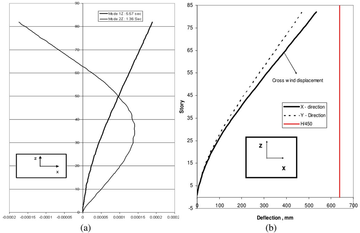
Figure 9:(a) 1<sup>st</sup> and 2<sup>nd</sup> translational mode; (b) deflection due to wind of the 82-story structure
