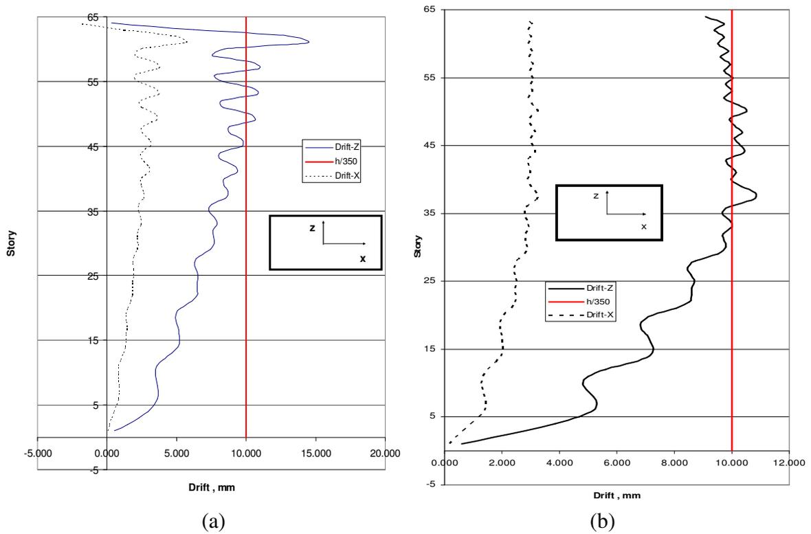
Figure 6: Inter-story drift of the 64-story structure due to wind from (a) Iteration-1; (b) Iteration-2
