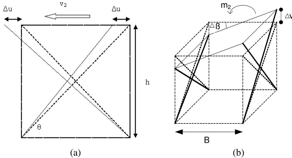
Figure 3: (a) Shear deformation of the module shown in Figure 2 – a portion of the web plane is shown; (b) Bending deformation of the module shown in Figure 2 – a portion of the flange plane is shown
