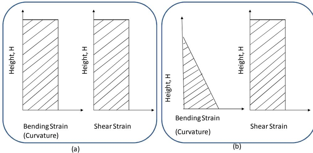
Figure 4: Shear and bending strain distribution along the height of the structure: (a) uniform curvature & shear strain distribution; (b) triangular curvature distribution & uniform shear strain distribution
