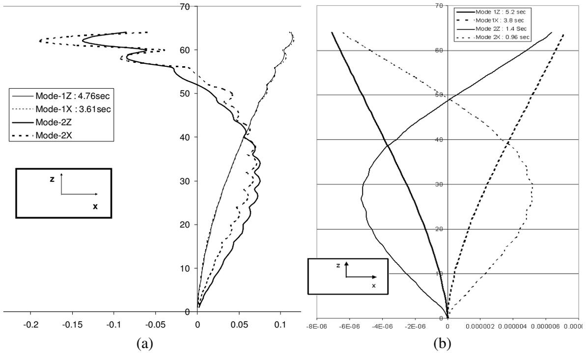
Figure 5: Mode shape of the 64-story preliminary structure of (a) Iteration-1; (b) Iteration-2
